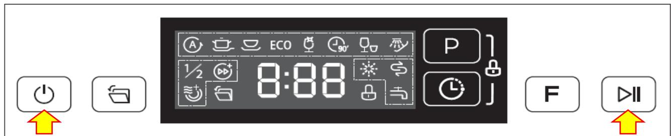
To access the test program, unplug then plug in the dishwasher
