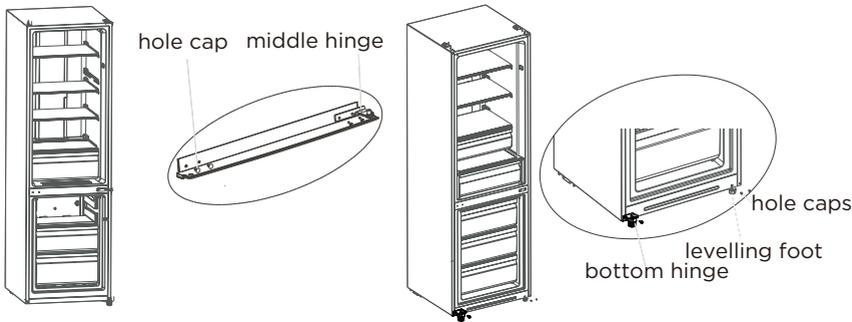
5. Dismantle the screws, sleeve pipe and stopper on the lower end cover of the two door bodies, and install them successively on the other side of the door bodies. Then remove the upper end cover of the cooler door and switch the wire harness with a sleeve pipe to the other side of the door body. Finally install the sleeve pipe of the upper hinge on the cooler door in the hole on the other side of upper end cover of the cooler door.
