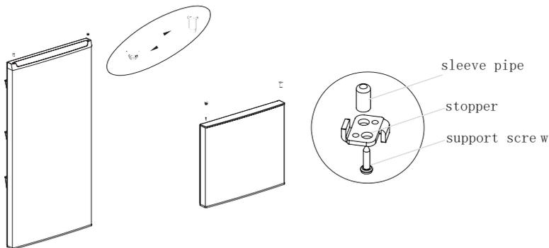
6. Put freezing door on bottom hinge and install middle hinge, hole caps
