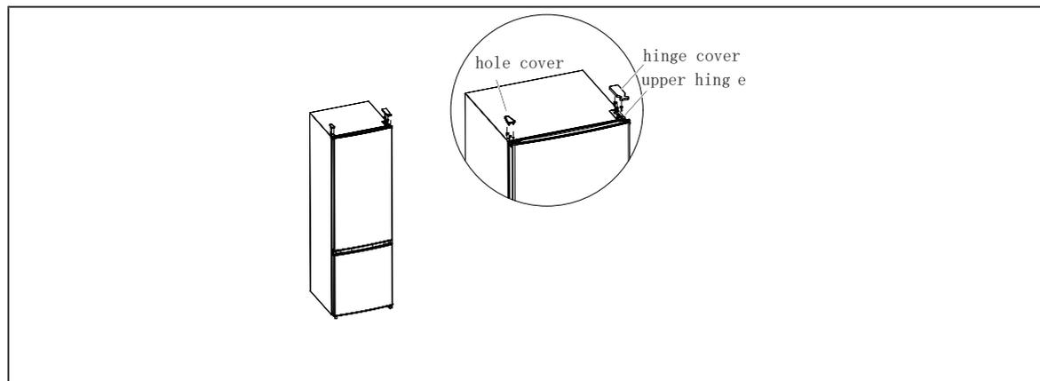
3. Take off refrigerating chamber door, middle hinge (use a cross screwdriver to remove the middle hinge screw) and hole cap of other side.
