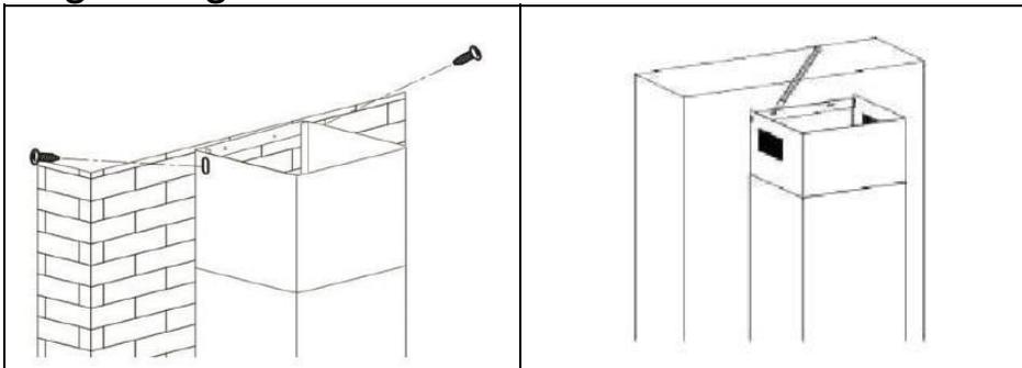
Step 10. Release the upper chimney and then drill holes on the wall.
