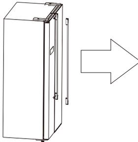
3. After the appliance is positioned, install the handles as reversed process.
