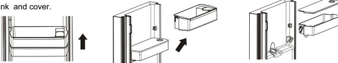
2. After cleaning, reposition water tank, cover and tank balcony as below process.
