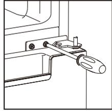
4. Laying down the refrigerator, take out the adjusting feet as below, then take off the lower hinge by cross screwdriver.
