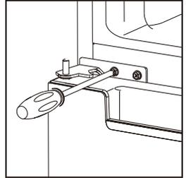
9. Place the upper door back on. Ensure the door is aligned horizontally and vertically so that the seal are closed on all sides before finally tightening the top hinge. Then insert the top hinge and screw it to the top of unit and then fix hinge cover (in accessory bag) by screw.
