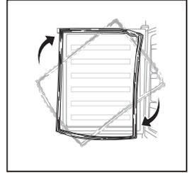
8. Install the lower door, adjust and fix the middle hinge onto the cabinet.
