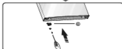
10. Change screw hole covers on middle cover plate from left to right (as shown in figure below).
