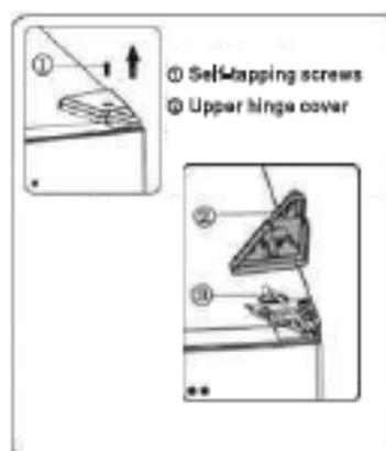
3. Remove screws ① and hinge ②. When the refrigerator with display on door, you need to pass connector ③ through the hole of hinge ②. (Please hold upper door by hand when installing).
