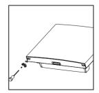
8. Make the middle hinge reverse the direction 180°C, then transfer it to the left property position. Make the middle hinge pin in the upper hole of the lower door, then tight the screws.
