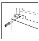
9. Install the upper door, fix the upper door hinge onto the cabinet and connect the wire.
