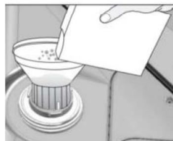
4. Fill the salt chamber of this machine with water only before the first use.
