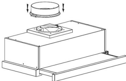
2. Mount the cooker hood on the cabinet by 6 screws (4×35mm) and flat washers.
