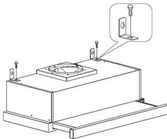
3. The cooker hood is wall mounted by 4 screws (4mm×30mm) and wall plugs.
