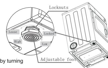
**Note** The locknuts must be tightened after adjustment. Any looseness can cause vibration and noise.
