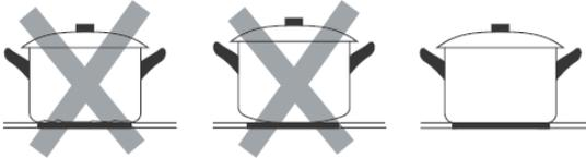
Make sure that the base of your pan is smooth, sits flat against the glass, and is the same size as the cooking zone. Use pans whose diameter is as large as the graphic of the zone selected. Using a pot a slightly wider energy will be used at its maximum efficiency. If you use smaller pot efficiency could be less than expected. Pot less than 140 mm could be undetected by the hob. Always centre your pan on the cooking zone.
