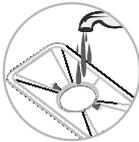
**A** Use flowing water to flush filter assembly. Do not use steel wool or iron brush, it will cause the filter rust.
