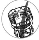
**B** Flush cylinder filter and filter net.
