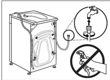
2. Connect the other end of the water supply hose to the water inlet valve on the rear of the appliance and tighten by hand.
