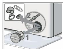
4. Reinstall the pump cover by screwing tightly into position. Handle must be vertically.
