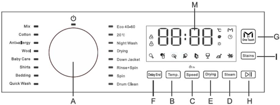
**A— WASH CYCLE SELECTOR knob:** Used to set the desired wash cycle (see “Table of wash cycles”).
