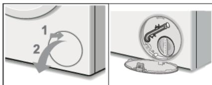
2. Pull the sealing cap from the emergency drain hose and lay the hose over the side of the basin and allow the water to finish draining from the drum.
