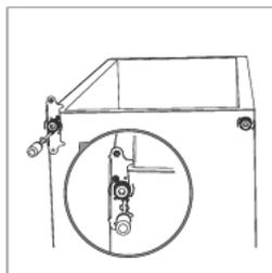
7. Place the upper door back on. Ensure the door is aligned horizontally and vertically so that the seals are closed on all sides before finally tightening the top hinge.
