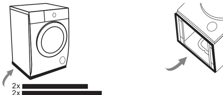
1. Get the machine laid on the floor, using some soft material like foam or clothes between the machine and floor for a protection.
