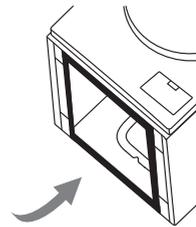
1. Get the machine laid on the floor, using some soft material like foam or clothes between the machine and floor for a protection.
