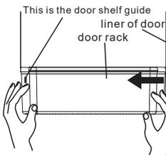
**Disassembly:** Hold both sides of the door rack with both hands. Push it from the side without the guide and push it inward as seen in the diagram. Push until the edge of the door rack is separated from the groove of the liner.
