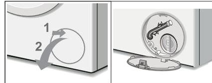
2. Pull the sealing cap from the emergency drain hose and lay the hose over the side of the basin and allow the water to finish draining from the drum.
