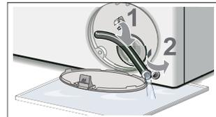
3. Turn the pump cover counterclockwise to remove it. A small amount of residual water may flow out when the cover is removed. Clean the interior of the pump housing, removing any debris or foreign objects. Check to be sure the impeller can now turn freely. Remove any lint, debris or detergent residue from the threads of the pump cover and the pump cover housing.
