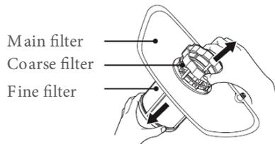
The fine filter can be pulled off the bottom of the filter assembly. The coarse filter can be detached from the main filter by gently squeezing the tabs at the top and pulling it away.
