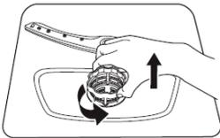
Hold the coarse filter and rotate it anticlockwise to unlock the filter. Lift the filter upwards and out of the dishwasher.
