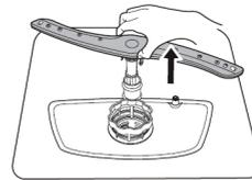
To remove the lower spray arm, pull out the spray arm upward.
