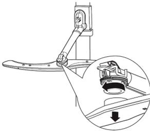
To remove the upper spray arm, hold the nut, rotate the arm clockwise to remove it.
