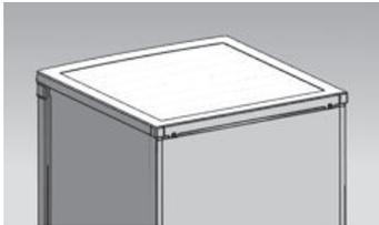
2. Remove the top hinge fixing screws with a cross-slot screwdriver. Take off the door and put it down carefully in a safe location.
