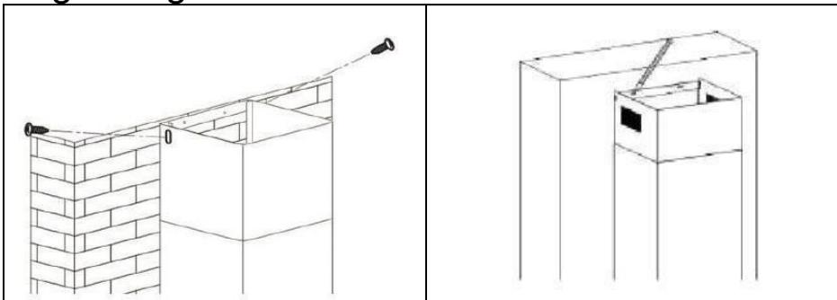
Step 10. Release the upper chimney and then drill holes on the wall.
