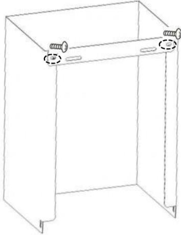
Step 5. Install the lower chimney on the appliance, and mark the holes position on the wall.
