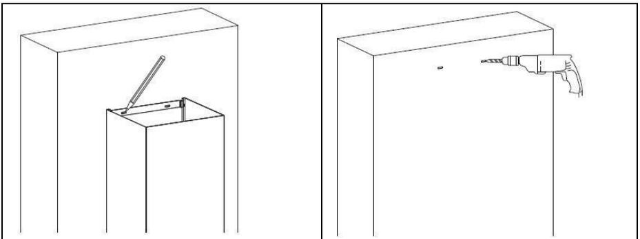
Step 7. Install the lower chimney on appliance again, then screw it to the wall with 2 screws of diameter  $\Phi$  4 mm and the corresponding wall plugs (not supplied). Also screw the chimney and the hood with 2 screws (ST4x8mm)
