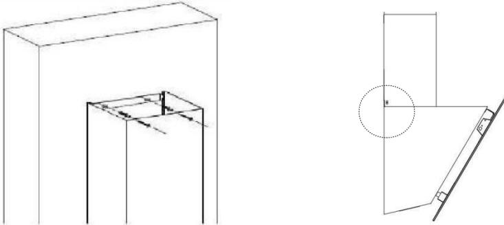
Step 8. Fix the upper chimney bracket on the upper chimney by 2 screws .ST4 x 8 mm
