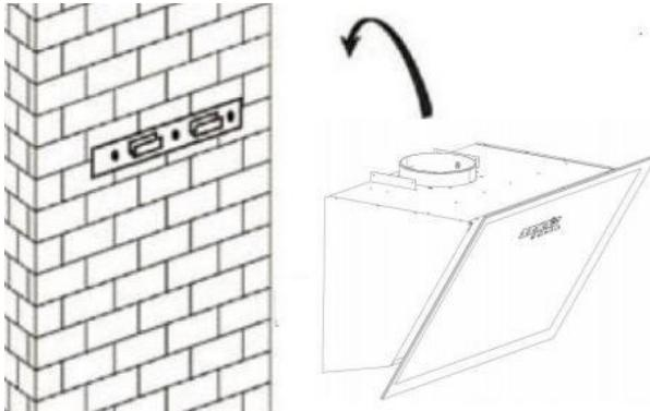
Step 3. (If the extraction installation mode is chosen) Place the  $\text{Ø}150\text{-}\text{Ø}153\text{mm}$  plastic pipe (supplied) on the air outlet as shown below. If the size of your plastic pipe is  $\text{Ø}120\text{ - } \text{Ø}123\text{mm}$  , you must firstly assemble the adapter to the air outlet, as shown below.
