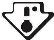
The following symbol shows the coolest zone in the refrigerator. This zone is between the fruit and vegetable glass shelf and the symbol, or the shelf located at the same height. To guarantee temperatures in this zone, do not modify the positioning of the shelves.
