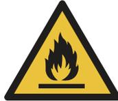
is a warning and indicates the refrigerant and insulation blowing gas are flammable.
