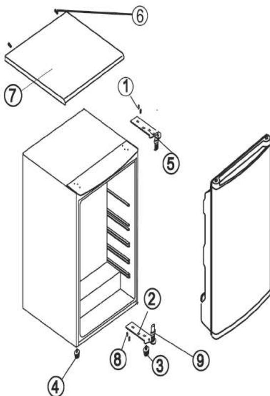
1. Remove the two screws. (6) securing the top. Remove the top (7).
