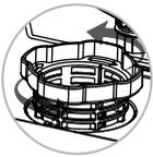
**A** Turn the cylinder filter out with anticlockwise.
