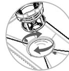
**C** You can put the filter back after cleaned. The cylinder filter should be assembled with clockwise until the triangle mark of filter, filter net and stainless steel in the same time.
