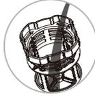
**B** Flush cylinder filter and filter net.
