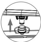
**A** Pull the main basket out of appliance, and lift the lower spray arm a little bit for loss the clips.
