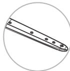
**B** Check if the spray arms blocked. If it does, please use a thin wire to pull the blockages out or flush the hole with water.
