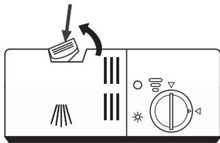
1. Press the release catch on the detergent dispenser to open the cover.
