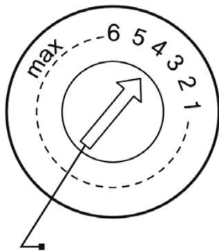
Turn the rinse aid indicator dial to a number between 1 and 6. The higher the number, the more rinse aid the dishwasher uses. If the dishes are not adjust lever drying properly or are spotted, adjust (Rinse) the to
