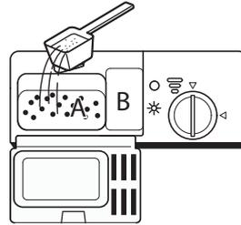
2. Add detergent into the larger cavity (A) for the main wash cycle. For more heavily soiled wash loads, also add some detergent into the smaller cavity (B) for the pre-wash cycle.
