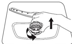
Hold the coarse filter and rotate it anticlockwise to unlock the filter. Lift the filter upwards and out of the dishwasher.
