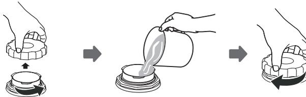
1. Remove the lower basket and unscrew the reservoir cap.
