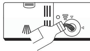
2. Carefully pour in the rinse-aid into its dispenser, whilst avoiding it to overflow.
