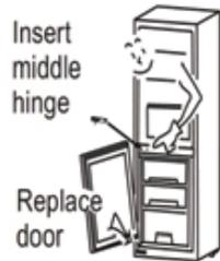
7. Place the fridge door on the middle hinge, making sure that the hinge pin is inserted in the hole at the bottom of the fridge door. Then put on the upper hinge, aim at the door and screw down the bolt, cover the left hinge cover and then screw down the bolt.
