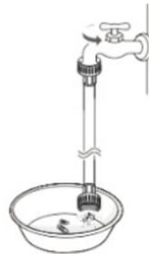
4. Connect the hose to the water inlet valve tightly by hand, and then tighten it for 2/3 turn with pliers.
