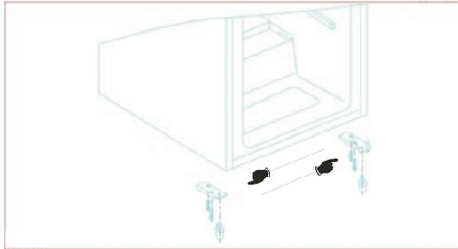
Unscrew the upper pin and screw it into place on the opposite side. Fit the door into the upper pin and close it. Screw the hinge pin bracket securely into place on the opposite side using the screws.
