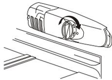
temperatures of around 25 °C, select setting 2. If you require a lower temperature, select setting 3 or 4.
