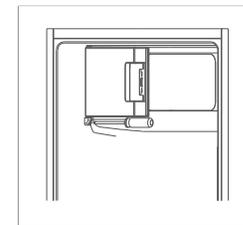
8. Unscrew the bottom hinge. Then remove the adjustable feet from both sides.
