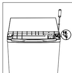
4. Unscrew the bottom hinge of the freezer door. Then remove the door and place it on a soft pad to avoid scratch.
