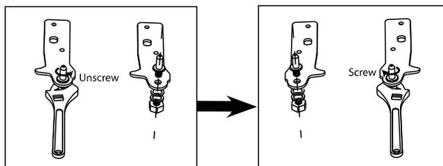
10. Replace the bracket that fits the bottom hinge pin. Replace both adjustable feet.
