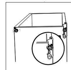
9. Unscrew and remove the bottom hinge pin, turn the bracket over and replace it.
