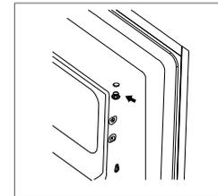
7. Rotate freezer door and place hinge side at left side. And then fix the door by holder.
