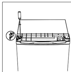
12. Put the top cover and fix it with 2 screws and then attach them after rotating.
