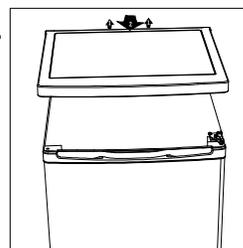
3. Unscrew the top hinge and then remove the door and place it on a soft pad to avoid scratch.
