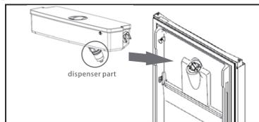
Pour water into the storage box part. Firstly, turn the cover of storage box anticlockwise and pull out the cover. Secondly, pour water into storage box, watching out the limit line. Lastly, covering the cover.
