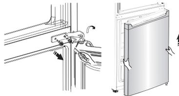
8. Place the lower door on a smooth surface with its panel upwards. Loosen screw 2 and part 1, then install them to the left side and tighten securely.
