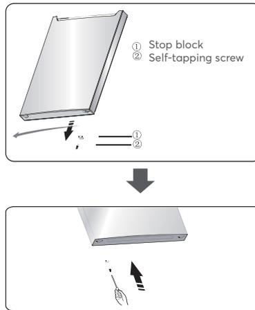
9. Change screw hole covers on middle cover plate from left to right (as shown in figure below).
