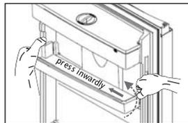
Press the right side of the door shelf inwardly, while holding the left side. When the notch of the shelf has been detached from the refrigerator door, remove the rack obliquely upwardly.
