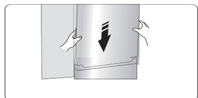
15. Transfer the upper hinge part and make the upper hinge axis into the upper hole of the upper door, and adjust the position of the upper door (please support the upper door with your hand when doing it), fixing the upper hinge part with the special flange self-tapping screws.
