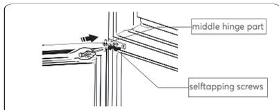
14. Transfer the upper door to the appropriate position. Secure the door's level, make the middle hinge axis into the lower hole of the upper door.
