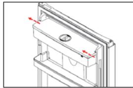
Install the water storage box part. Put the dispenser part into the hole of the door. Align the door liner, then press in the water storage box toward thirty degrees below the horizontal plane.
