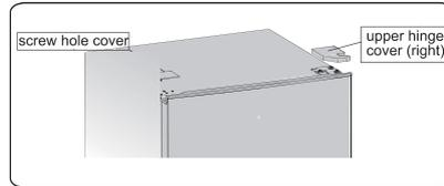
3. Unscrew the special flange self-tapping screws which are used for fixing the right upper hinge part by a 8mm socket driver or a spanner (please support the upper door with your hand when doing it) .
