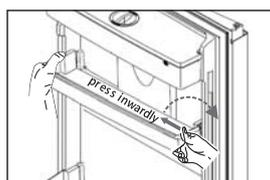
Firstly tilt the left side of the door shelf, and make sure the notch has been fastened to the door. Then press the right side inwardly, push it down to the right place. Remove the water storage box part. Pull out the water storage box toward thirty degrees above the horizontal plane.
