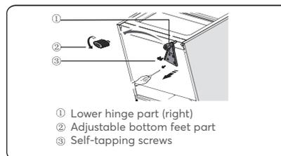
11. Replace the lower hinge part to the left side and fixing it with the special flange self-tapping screws. Replace the adjustable bottom feet parts to another side and fixing it .
