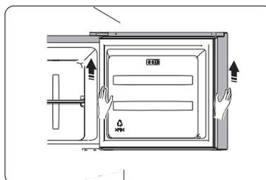
6. Place the upper door on a smooth surface with its panel upwards. Loosen screw 2 and part 1, then install them to the left side and tighten securely.
