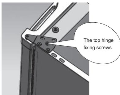
3. Place the top hinge, bushing and door stop on the other side.
