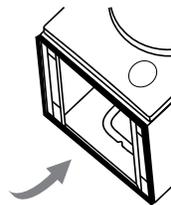
1. Get the machine laid on the floor, using some soft material like foam or clothes between the machine and floor for a protection;
