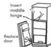
7. Place the freezer door on the middle hinge, turn over the top hinge to fix the top of the freezer door. Finally refit the top cover and install the plastic decorative piece into the right of the top cover
