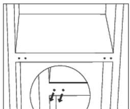
11. Stand up the unit and put the door on the bottom hinge. Make sure the bottom hinge core is inserted in the door hole. Then move the hinge hole cover of bottom door from left side to right side.
