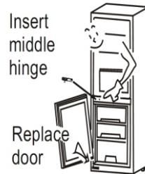
7. Place the fridge door on the middle hinge, making sure that the hinge pin is inserted in the hole at the bottom of the fridge door. Aim at the door and screw down the bolt, pull back the top cover from the front to the back, insert it in the top cover from side to side and screw down the two bolts of the back of the top cover.
