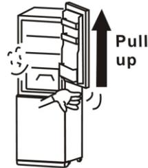
3. Using a screwdriver, dismantle the middle hinge. Lift the door upwards to disengage it from the lower hinge. Put the door to one side and lay it down gently on a padded surface.
