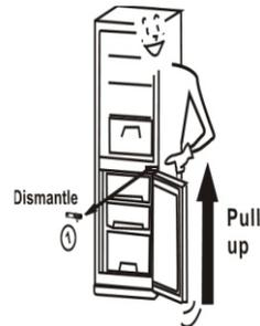
4. Swap over the position of the lower hinge and the adjustable leg to the other side of the cabinet.
