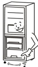
5. Remove the hinge pin that is in the bottom of the fridge and freezer door. At the other side of the fridge and freezer door, insert the replacement hinge pin that is supplied with the appliance.
