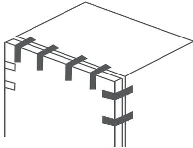
2) Dismantle hole caps, the upper hinge cover, fitting screws of upper hinge, and remove the upper hinge, please keep the door vertical in whole process for avoiding falling down;
