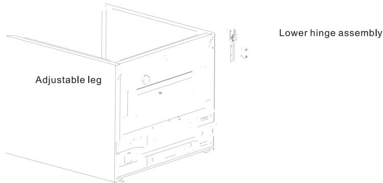
5) Install the lower hinge and adjustable leg on lower left side of cabinet and lower right side respectively;
