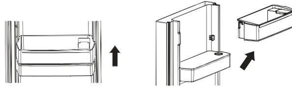
2. Remove the water tank. Detach the top cover and wash and clean both the tank and the cover.
