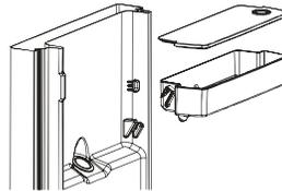
3. After cleaning, reposition water tank, cover and tank balcony as below:-
