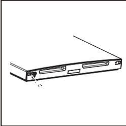
9. Install the lower door, adjust and fix the middle hinge onto the cabinet.
