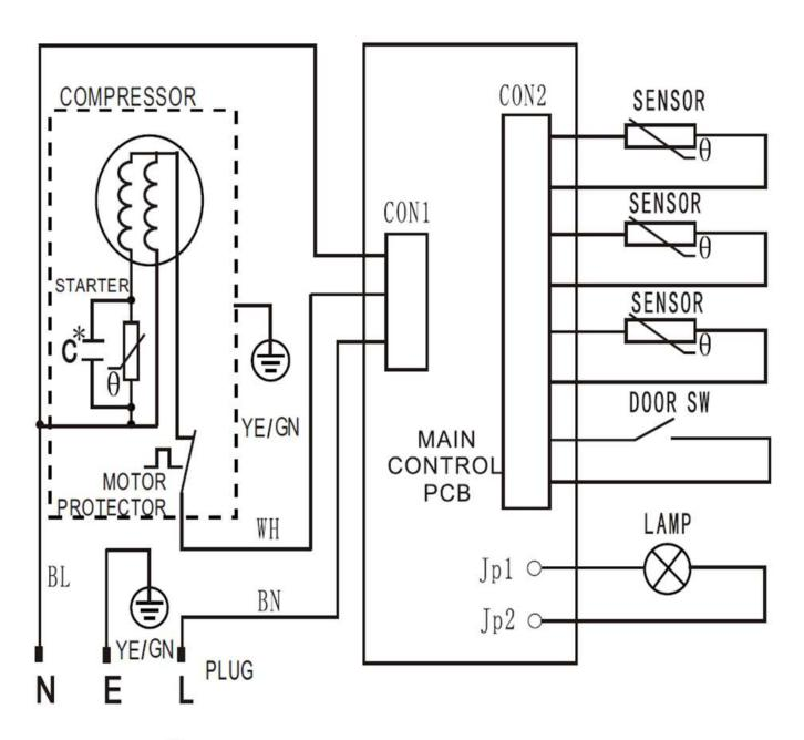
**C\***:The capacitor is optional according to different compressor model
