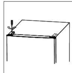
14. Fix the hinge cover on the left and the hinge hole cover on the right.
