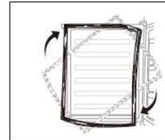
9. Make the middle hinge reverse the direction, then transfer it to the left property position. Make the middle hinge pin in the upper hole of the lower door, then tight the bolts.
