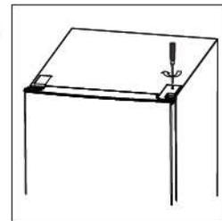
2. Unscrew and remove the hinge.
