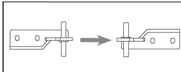
10. Place the upper door back on. Ensure the door is aligned horizontally and vertically so that the seal is closed on all sides before finally tightening the top hinge. Then insert the hinge and screw it to the front of the unit.
