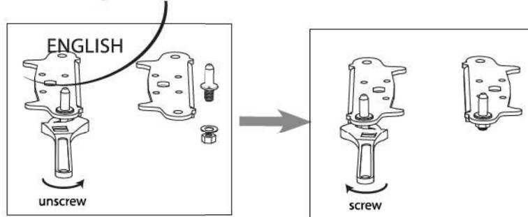
7. Refit the bracket fitting the bottom hinge pin. Replace both adjustable feet. Transfer the lower door to the property position.
