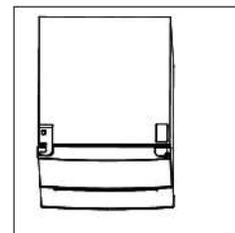
11. Unscrew the hinge pin and reverse the hinge, then reinstall the hinge pin.
