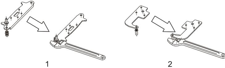
6. Install the lower hinge under the refrigerator like below, screwing in the adjusting feet, make sure the position in horizon.
