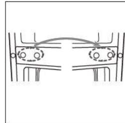
6. Unscrew the bottom hinge. Then remove the adjustable feet from both sides.
