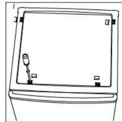
2. Unscrew the top hinge and then remove the upper door and place it on a soft pad to avoid scratches.
