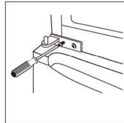
11. Place the upper door back on. Ensure the door is aligned horizontally and vertically so that the seal are closed on all sides before finally tightening the top hinge. Then insert the hinge and screw it to the top of the unit.
