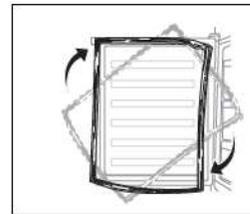
10. Reverse the middle hinge at 180°, then transfer it to the proper position at the left side. Put the middle hinge pin in the upper hole of the lower door, then tighten the bolts.
