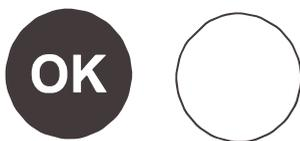
If the indicator of temperature turns WHITE, this means that the temperature is too high; in this case, increase the refrigerator temperature control setting and wait for 12 hours before performing a new visual inspection of the indicator.
