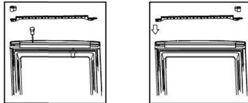
3. Unscrew from the middle hinge by cross screwdriver, then take off the lower door.
