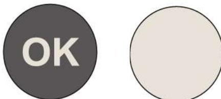
If the indicator of temperature turns WHITE, this means that the temperature is too high; in this case, increase the refrigerator temperature control setting and wait for 12 hours before performing a new visual inspection of the indicator.
