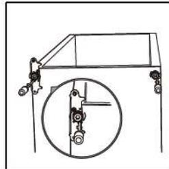
7. Unscrew right middle stopper with metal block from bottom of upper door. And then install left middle stopper and metal block in left side of bottom of upper door.
