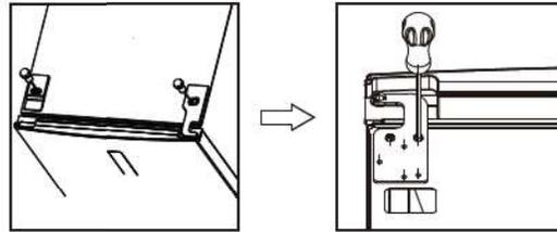
2. Please upwarp and take off plastic cover and wire sleeve by straight screwdriver. Please be careful of the wire inside. Then move wire with connector to another side and install wire sleeve to another side and fix cover back.
