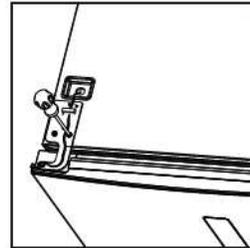
10. Take left hinge cover from accessory bag and install it with top hinge. Then install hole cover at right side.
