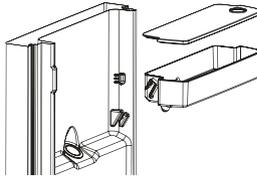
3. After cleaning, reposition water tank, cover and tank balcony as below:-
