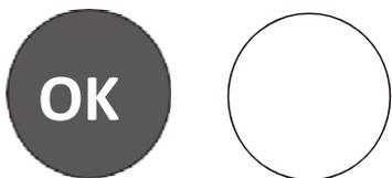
If "OK" does not appear, the temperature of the zone is too high. Set the thermostat to a higher position. Wait at least 12 hours before readjusting the thermostat. After loading fresh food into the appliance or after repeated openings (or extended opening) of the door, it is normal for the temperature indicator not to display "OK".
