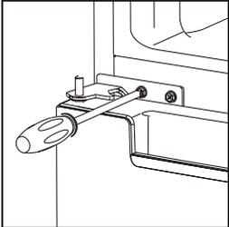
9. Place the upper door back on. Ensure the door is aligned horizontally and vertically so that the seal are closed on all sides before finally tightening the top hinge. Then insert the top hinge and screw it to the top of unit and then fix hinge cover (in accessory bag) by screw.
