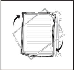
8. Install the lower door, adjust and fix the middle hinge onto the cabinet.
