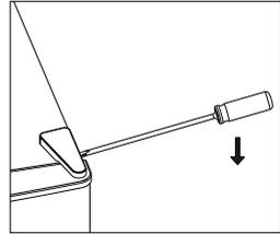
2. Unscrew the top hinge with a philiphs screw driver.
