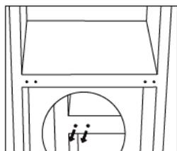
7. Lie down the rear of cabinet on a soft pad. And unscrew the bottom hinge and leveling foot.
