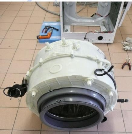
Remove the axles from the shock absorbers and remove the hose at the level of the drain pump.
