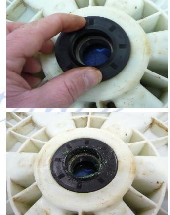
Position the inner bearing, knock to push it against the hub: when knocking, the "dull" noise becomes "metallic".
