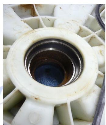
After changing the disc diameter, position the bearing punch to extract both the inner bearing and the oil seal.
