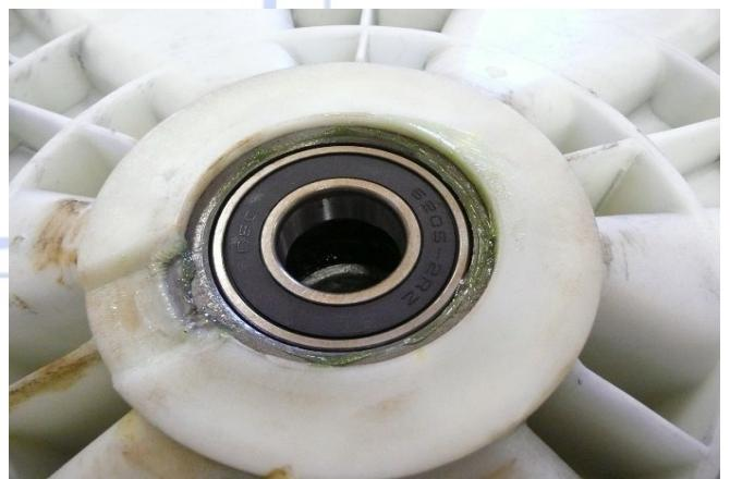
Position the outer bearing, knock to push it against the hub: when knocking, the "dull" noise becomes "metallic".
