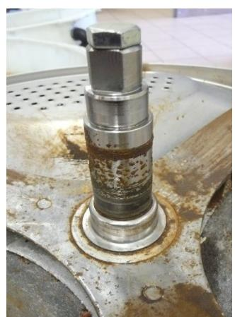
Apply penetrating oil to the crosspiece and leave to act for a few minutes. Place the cleat on the pulley screw, strike with the hammer to remove the drum.
