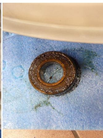
Remove the outer bearing using the bearing puller. Position the half-tank on 2 wooden cleats so as not to damage it.
