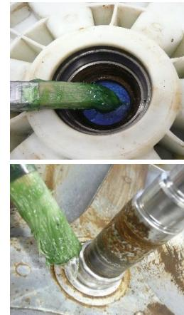
Replace the tank seal to prevent any water leaks.
