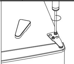
A line drawing showing a cross screwdriver being used to unscrew the top hinge. A triangular cover is shown separately to the left.                                                  |
