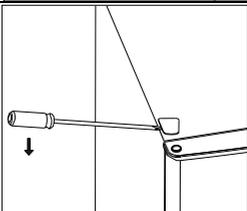
A line drawing showing a flat screwdriver being used to pry off a small rectangular cover from the opposite side of the hinge. A downward arrow indicates the direction of the pry. |
