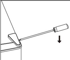
A line drawing showing a flat screwdriver being used to pry off a triangular cover from the top hinge of a door. A downward arrow indicates the direction of the pry.                 |
