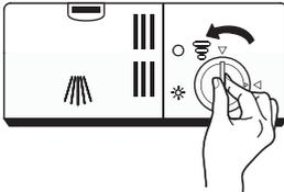
1. Remove the rinse aid reservoir cap by rotating it counter clockwise.
