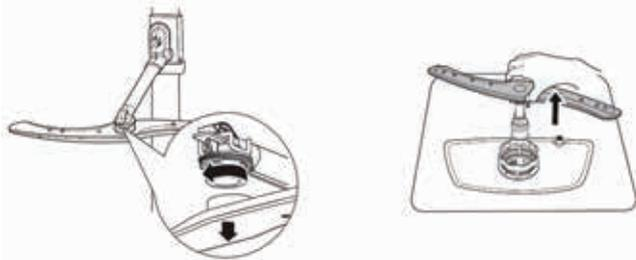
To remove the upper spray arm, hold the nut, rotate the arm clockwise to remove it.
