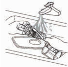
Larger food remnants can be cleaned by rinsing the filter under running water. For a more thorough clean, use a soft cleaning brush.
