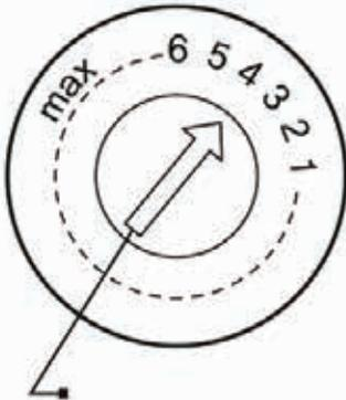
Turn the rinse aid indicator dial to a number between 1 and 6. The higher the number, the more rinse aid the dishwasher uses. If the dishes are not adjust lever drying properly or are spotted, adjust (Rinse) the to the next number until your dishes are spot-free. Reduce it if there are sticky whitish stains on your dishes or a bluish film on glassware or knife blades.
